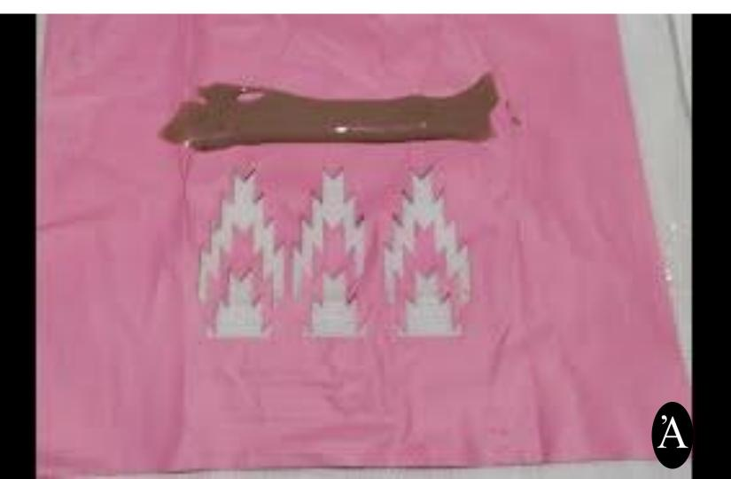
At the end, the print was very good, the problem with the run off is due to the manipulation and construction of the screen
