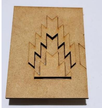
I made an MDF cut seal with the laser cutter to test the ink. It can be improved but I think it is a good solution to avoid run off of the dye.
