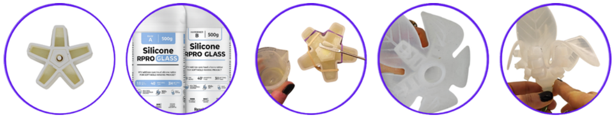
Silicone pneumatic actuator fabrication workflow, from mould preparation and silicone mixing to demoulding, scaffold connection and inflation testing. Carlotta Premazzi, 2026.
