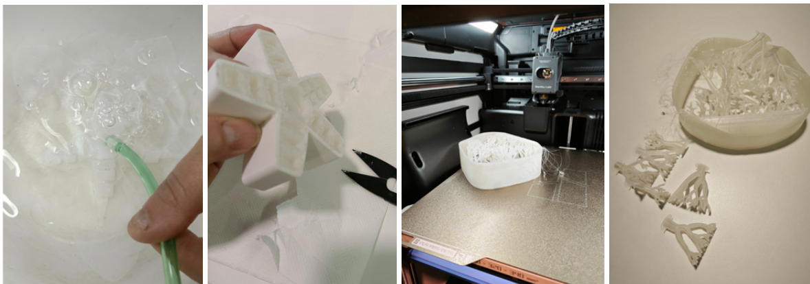
Challenges and failures during fabrication, including air bubbles, blocked pneumatic channels, excessive support material and loss of detail in organic branching elements. Carlotta Premazzi, 2026.
