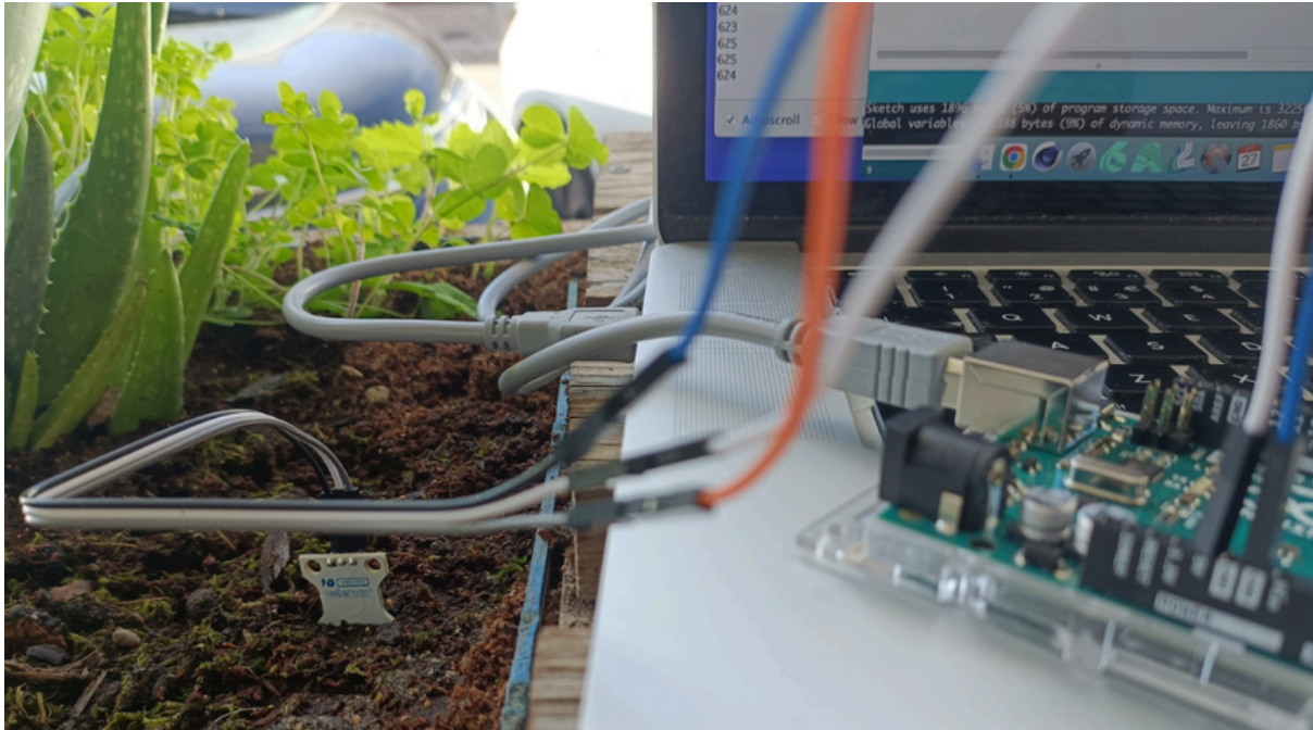
Resistive Soil Moisture Sensor testing. Carlotta Premazzi, 2026.
