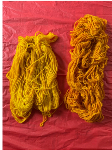
Figure 10. Comparison of turmeric-dyed wool yarn samples, showing color variation produced through different mordants and modifiers.
