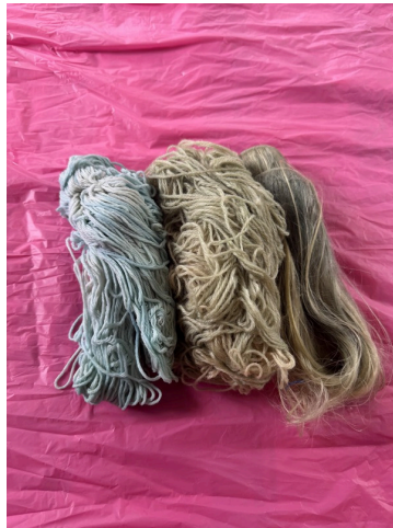
Figure 13. Naturally dyed yarn and hair samples produced from black bean dye experiments, demonstrating color variation across different materials.
