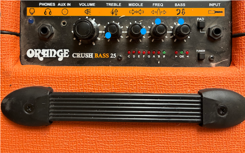
Bass Amplifier Settings (blue dots indicate where to turn the knob)
