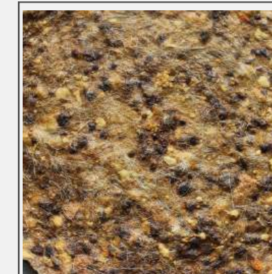
Rain water Alginat: 85g Washed wool: 2g Orange filler: 15g
