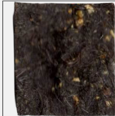
Rain water Alginat: 211g Washed wool: 6g Orange filler: 6.20g
