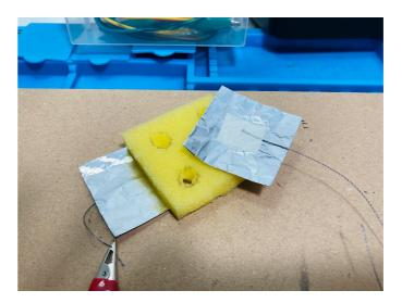
Aluminium foil Tape Conductive thread Foam with holes
